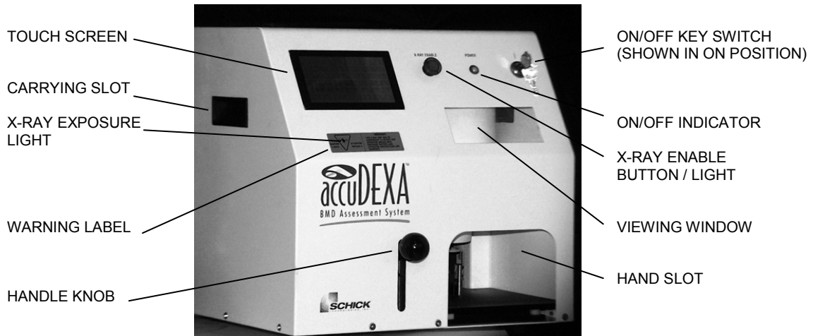
Figure 1. The accuDEXA Device, front view
